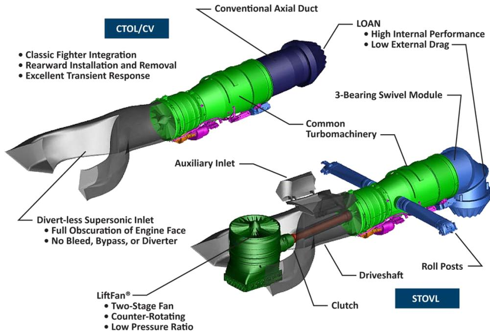
**Fig. 17 Comparison of F-35 conventional and F-35B STOVL lift systems.**
