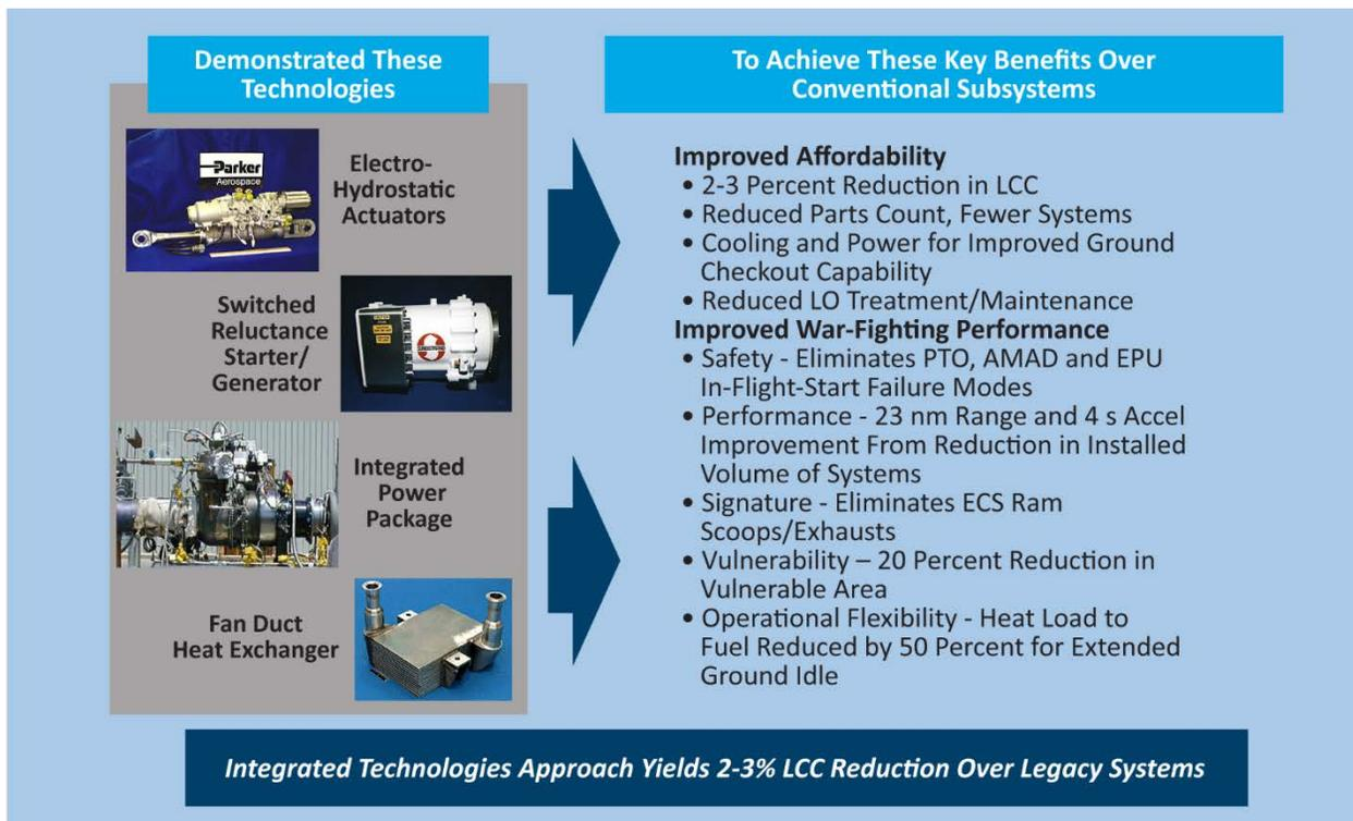
Fig. 4 Benefits of integrated subsystems technologies.
