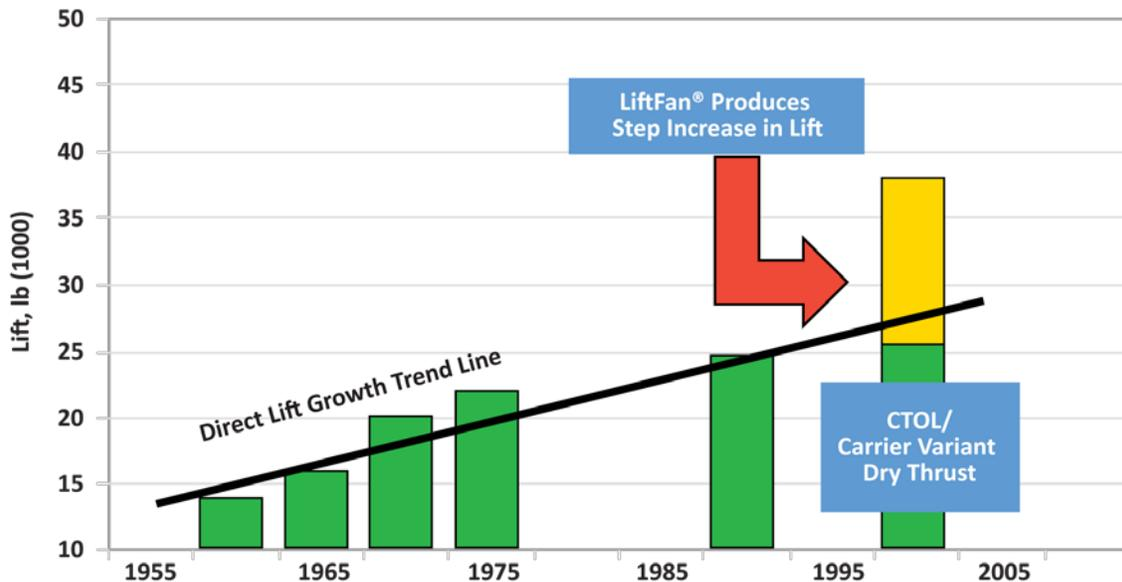
Fig. 16 Revolutionary step increase in vertical lift.
