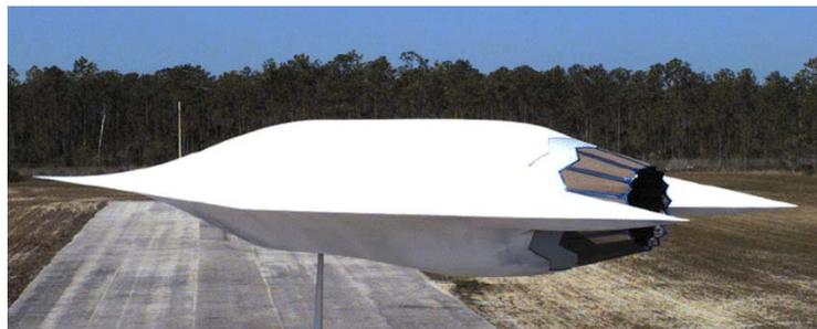
**Image 4 Radio frequency test fixture with the F-35 LO nozzle at the Pratt & Whitney facility in West Palm Beach.**
