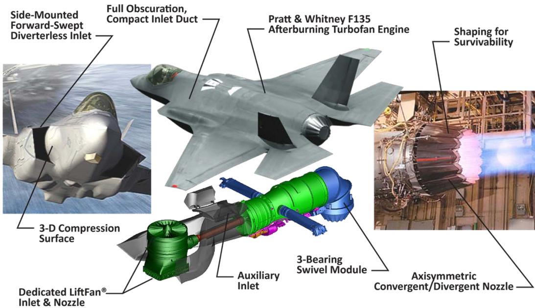
**Fig. 11 F-35 advanced propulsion system technologies.**
