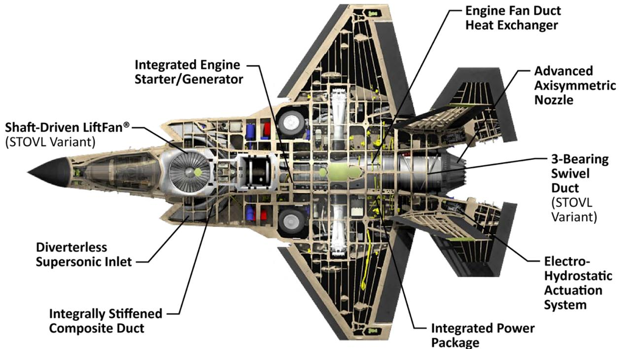
**Fig. 1 Advanced technologies selected for F-35 air vehicle and propulsion systems incorporation.**
