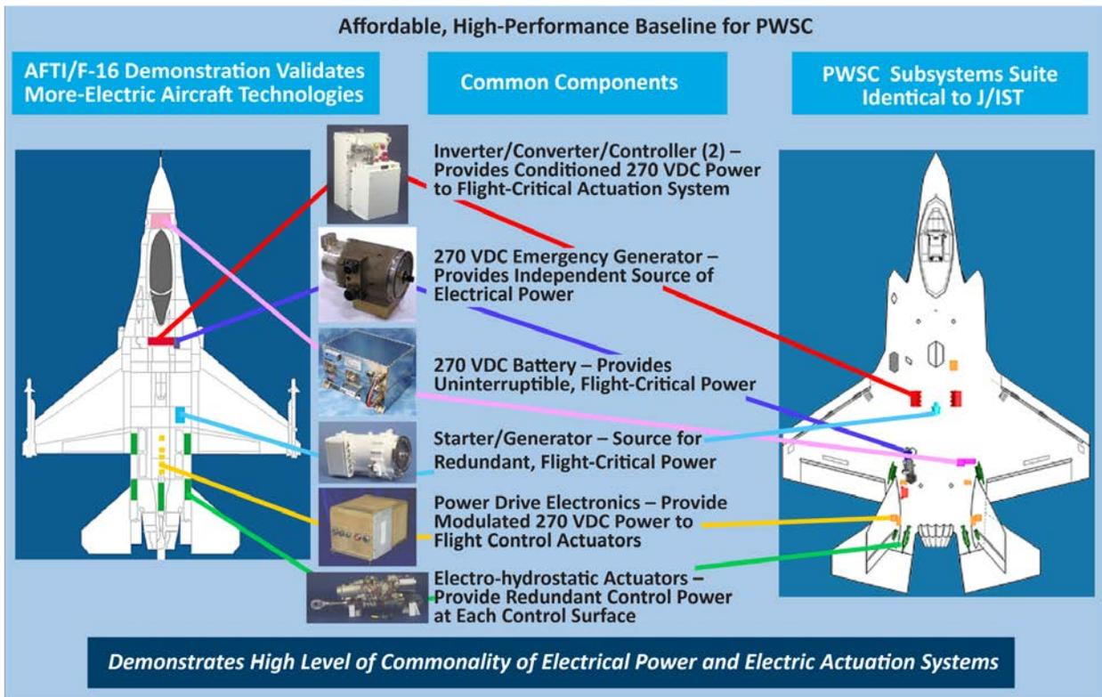
**Fig. 5 AFTI/F-16 J/IST aircraft MEA technologies and transition to F-35.**
