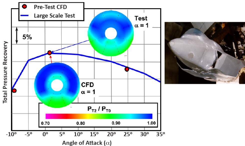
**Fig. 14 Large-scale wind tunnel testing validation of CFD design methodology and CFD test model (inset).**
