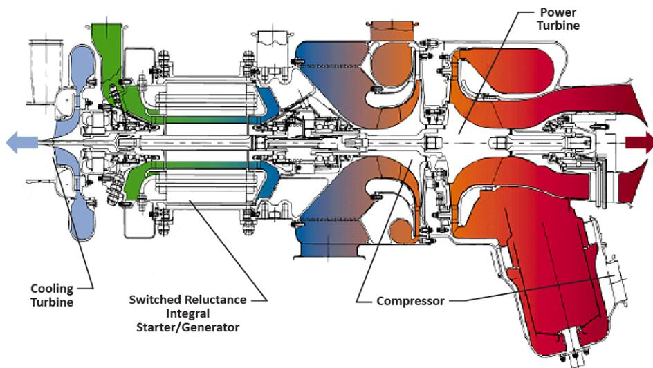
**Fig. 9 T/EMM turbomachine cross-section.**
