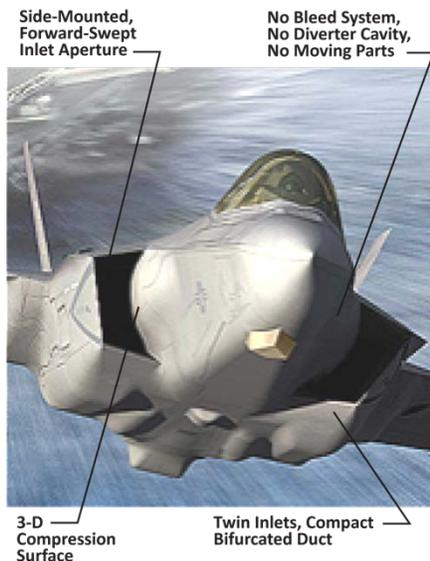
**Fig. 12 F-35 engine air induction system features.**
