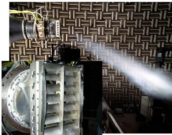
**Image 5 Twenty-seven-percent-scale F-35B STOVL VAVBN test, with (inset) VAVBN closeup.**
