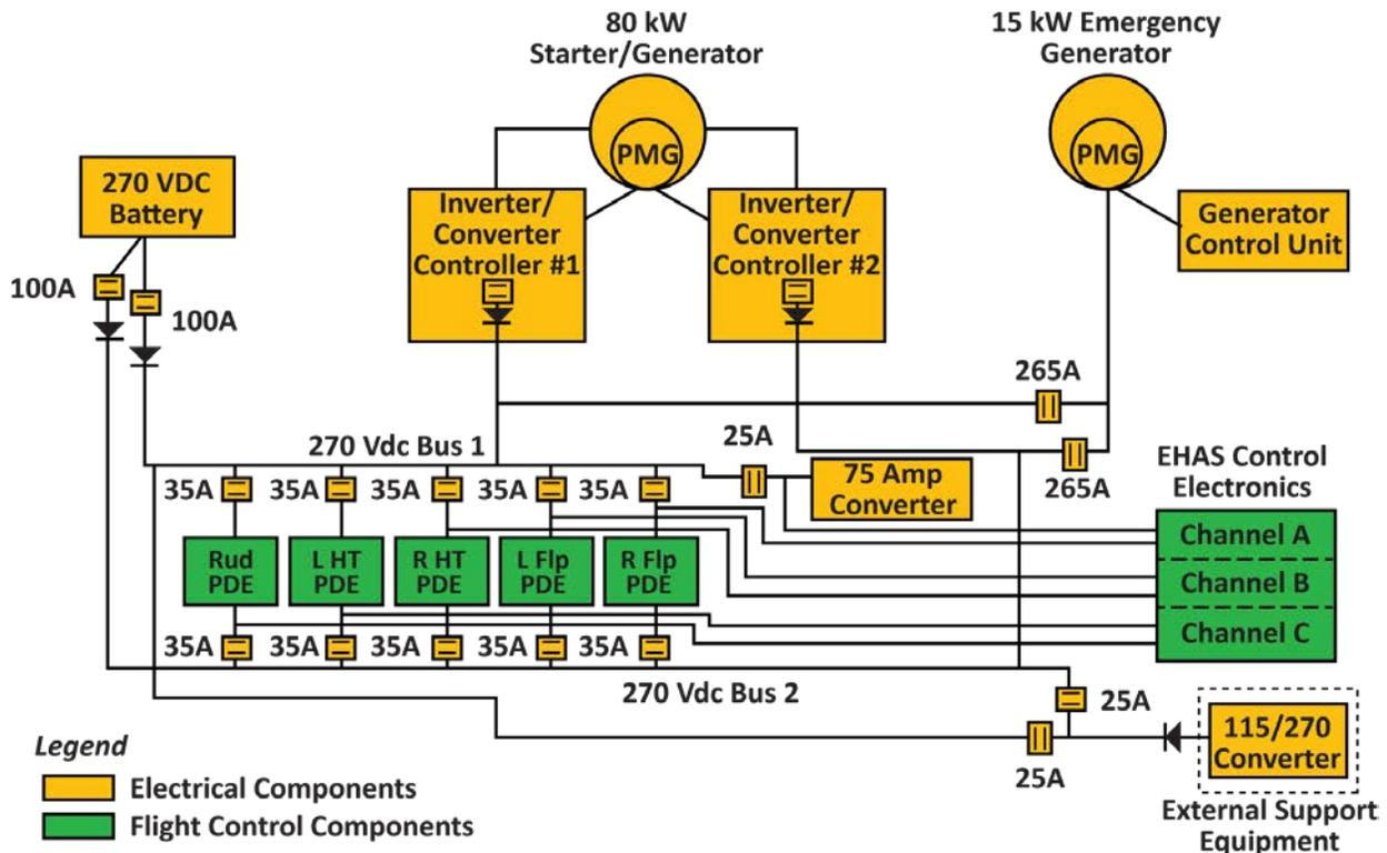
**Fig. 6 AFTI F-16 J/IST electrical power and actuation flight demonstration architecture.**
