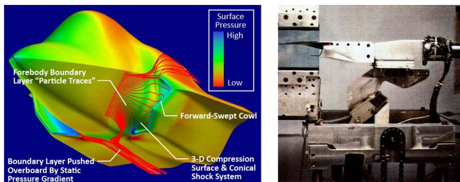
**Fig. 13** CFD simulation of DSI supersonic boundary layer diversion.
