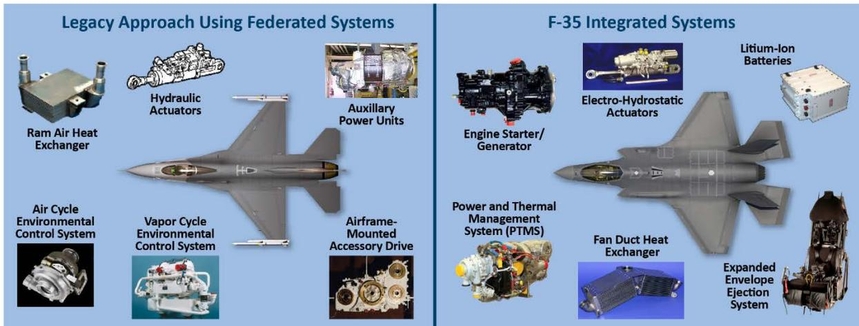
Fig. 3 F-35 integrated vehicle systems.
