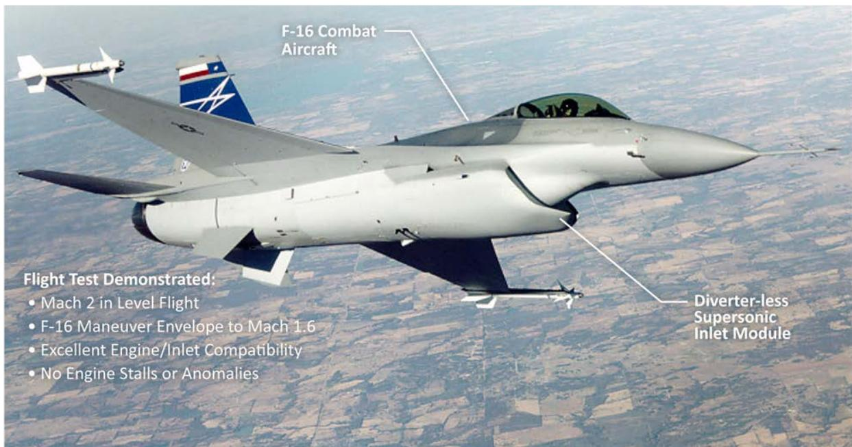
**Fig. 15 DSI technology was matured through rigorous F-16 flight demonstration.**
