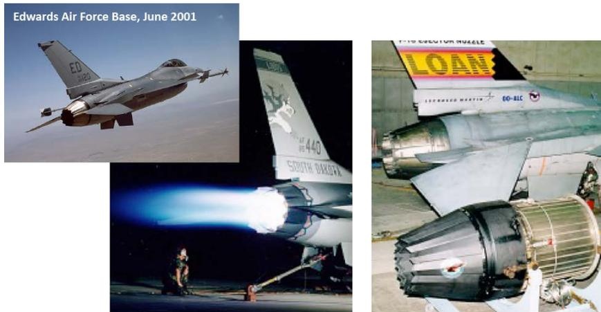
**Image 3 General Electric LO Axi Nozzle (left) and Pratt & Whitney LOAN (right) ground and flight testing on the F-16.**
